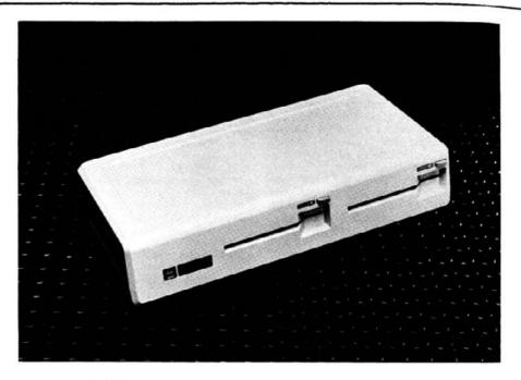
Duofile provides Apple III users with an additional mass storage alternative. It contains two of Apple's new 871 disk drives, with a capacity of 871, 424 bytes per disk drive, thus providing built-in backup.
